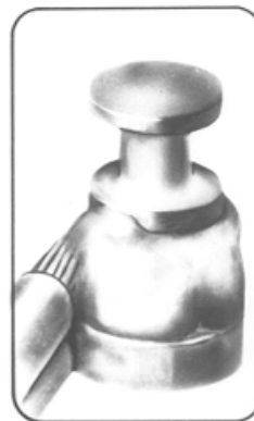
Unacceptable Excessive solder
