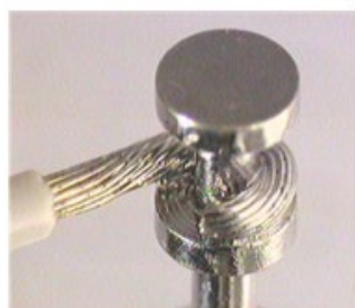
Unacceptable Insufficient solder joint
