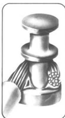
Unacceptable Insufficient solder
