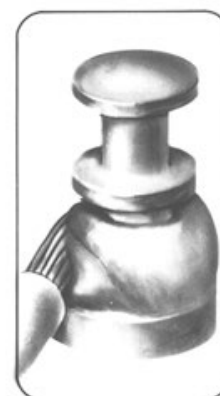
Unacceptable Excessive solder
