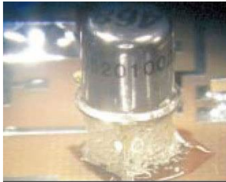
Figure 8-2: TO package with underfill
