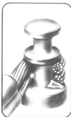
Unacceptable Insufficient solder
