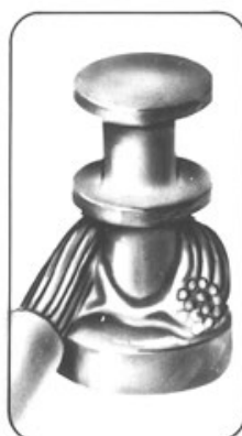
Acceptable Minimum solder
