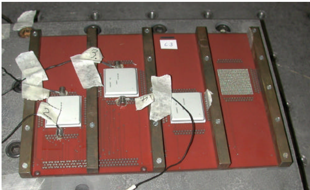
Figure 23. View of a test board with via-in-pad design mounted on the vibration exciter
