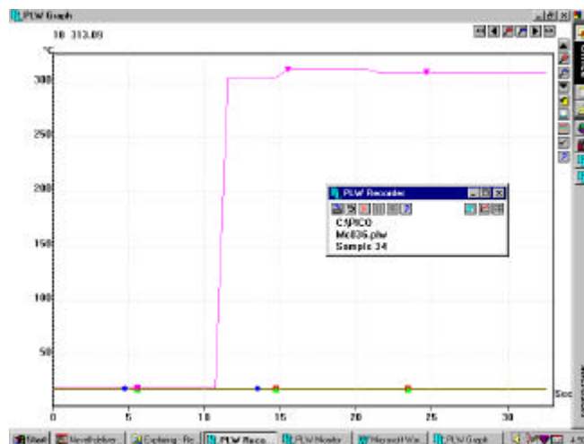
Graph A-2-2: Metcal 036 No Load Peak Temp 313°C (nominal 315°C)
