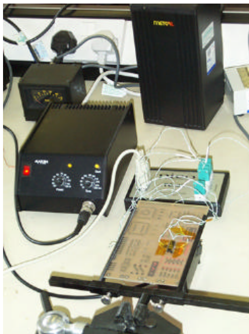
Fig 5.1-1b: The Martin IR Lamp is positioned under the board with thermocouples in place.
