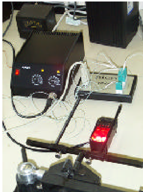
Fig 5.1-1a: The Martin IR Lamp is positioned under the board holder.
