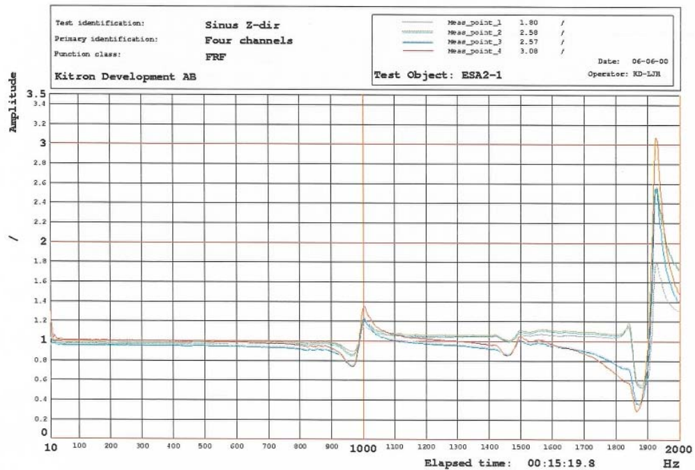
Figure 15. Acceleration recorded during the sine vibration test in the x-direction (upper diagram) and in the z-direction (lower diagram) for the board with EPO-TEK 930 applied beneath the components
